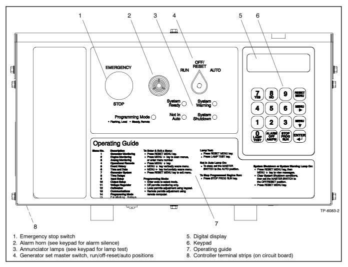
Figure 1-1 550 Controller with Three-Position Selector Switch
